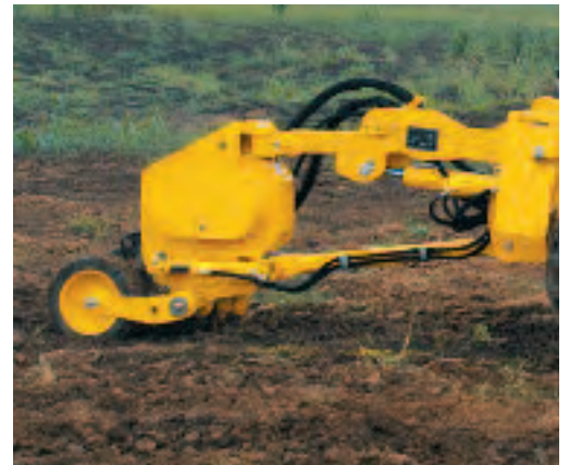
Vibratory plow. When teamed with the quad-track system, the plow is capable of reaching depths up to 36" (91.4 cm).
