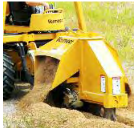
Rockwheel. Rugged construction for depths up to 26" (66 cm) at 6" (15.2 cm) wide.
