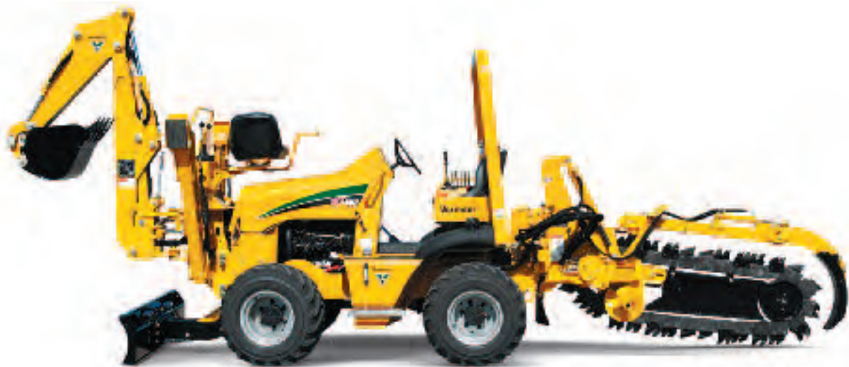
Trencher. Available in a center-mount or sliding-offset configuration, the trencher is capable of depths reaching 60" (152.4 cm) and widths up to 12" (30.5 cm).
